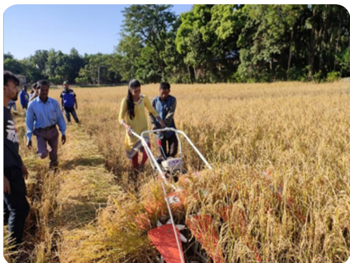
User friendly Reaper being used in the paddy fields to harvest paddy
