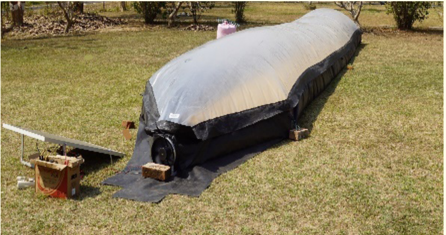
Solar bubble dryer
